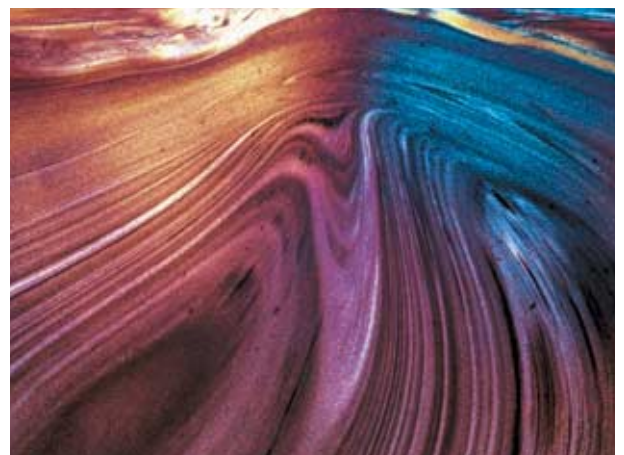
Polyethylene cold melt, Nz.temp. staining, polarized light with first-order red compensator, original scale 10:1
