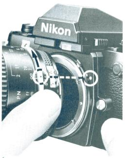
Grasp the lens by its mounting ring. Position the lens in the camera's bayonet mount, lining up the aperture index on the lens with the lens mounting index on the camera, and twist the lens counterclockwise until it clicks into place.
