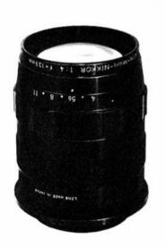
136mm Focal length f/4 Max. aperture Construction 7 elements, 4 groups 1/25X Standard magnification 20° at f/4, 25.5° at f/5.6 Pícture angle 3.640mm Overall working distance 1,250mmø (at f/4) Object area 1,600mmø (at f/5.6) Image area 50mmø (at f/4)
