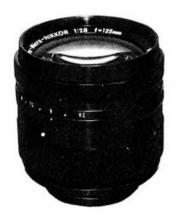
Focal length 125mm Max. aperture f/2.8 Construction 7 elements, 6 groups Standard magnification 1/25X 12.3° Picture angle 3,364mm Overall working distance Object area 700mmø 28mmø Image area Standard wavelength 546mu (e-line) Aperture efficiency at image corner 100% at f/2.8 (no vignetting) Distortion Aerial resoving power 400 lines/mm Aperture scale 2.8.4.5.6.8 Mount Screw d=62mm p=1mm Adapter plate o.d.=77.5mm Dimensions: max. diameter 81mm max. length 86mm
