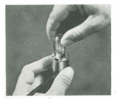
Press the **6-volt**, **15-watt lamp**, 38 01 77, down into the socket (red dot facing red pin) and lock it by clockwise rotation. Wipe fingerprints from the glass bulb to avoid their burning in and slip the black sleeve serving as glare shield over the bulb.
