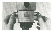
The focal length of the zoom lens can be varied continuously. Every change in the position of the revolving nosepiece is equivalent to a change in magnification on the film by the factor 4.
